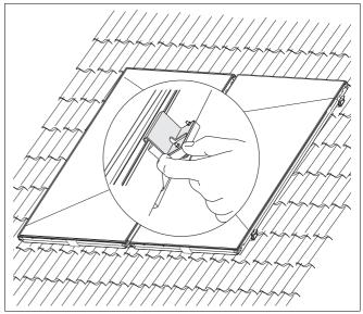
Fig. 37 Securing collectors to the side
