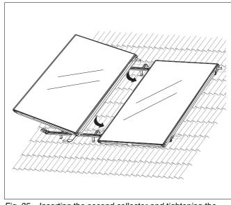
Fig. 35 Inserting the second collector and tightening the hose clip
