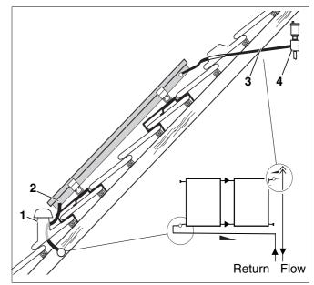
Fig. 44 Position of air vent with bleeder
