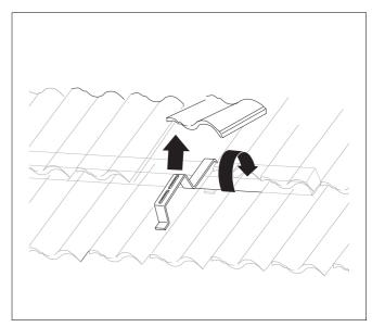
Fig. 21 Attaching roof hooks
