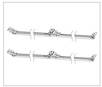
Fig. 11 Preassembled profile rails for two adjacent collectors
