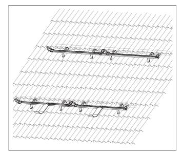
Fig. 17 Profile rails with roof hooks installed on a tile roof – for two adjacent collectors
