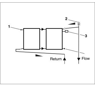
Fig. 39 Water connection acc. to the Tichelmann principle
