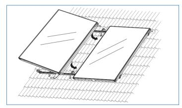
The second panel (of a two panel array) can be added easily with push-fit connections.
