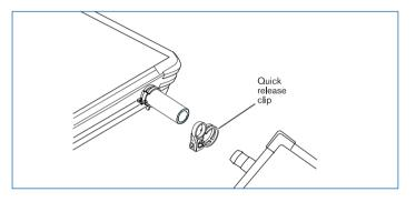
Subsequent collectors in series also use this connection method to enable arrays to be plumbed-in with ease.
