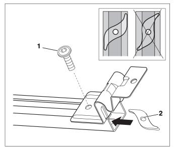
Fig. 15 Securing the collector holder flush with the profile rail **Item 1:** Pan-head screw (M8 x 16, preassembled)
