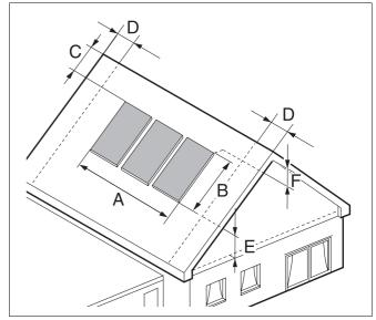
Fig. 10 Space required for collector array
