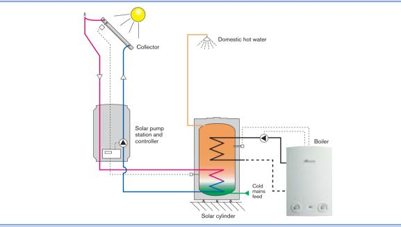
The most common solar system layout uses a twin coil cylinder which is fed by both a boiler (or other heat source) and the solar panels. The solar system and the regular heating system do not come into direct contact with each other and the only shared part is the cylinder.
