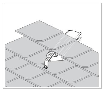
Fig. 30 Special roof hook fully installed
