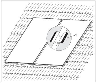
Fig. 36 Securing collectors centrally
