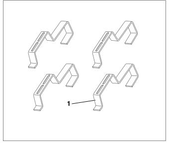
Fig. 5 Roof hook installation set
