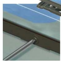
Tops are secured or removed using the two locking fasteners on the leading edge.
