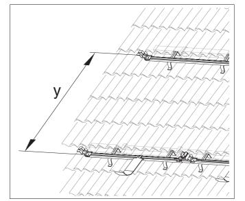
Fig. 19 Distance of the profile rails from one another
