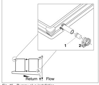
Fig. 45 Dummy plug installation
