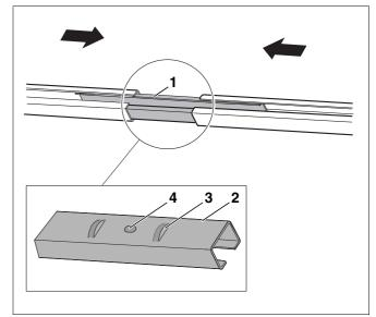
Fig. 12 Plugging profile rails together
