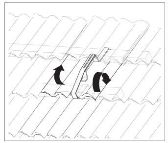
Fig. 22 Attaching additional roof hooks
