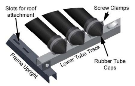
**Uprights:** Run the full height of the collector and are used for attachment to the mounting surface (roof, wall). Slots are punched out along the length for the attachment of mounting straps (stainless steel 'builders strap' is ideal ). Additional brackets/holes may be made according to your specific mounting requirements. The width between uprights is adjustable to suit individual installation requirements.
