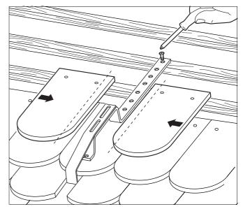
Fig. 29 Cutting and installing crown tiles
