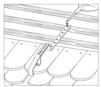
Fig. 28 Installing special roof hooks
