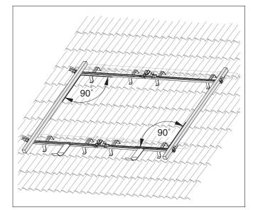
Fig. 24 Aligning profile rails
